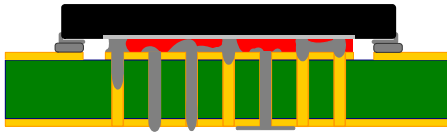
Figure 11. Solder Voiding Due to Solder Wicking
